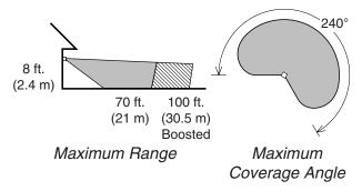
The detector is less sensitive to motion directly towards it.
